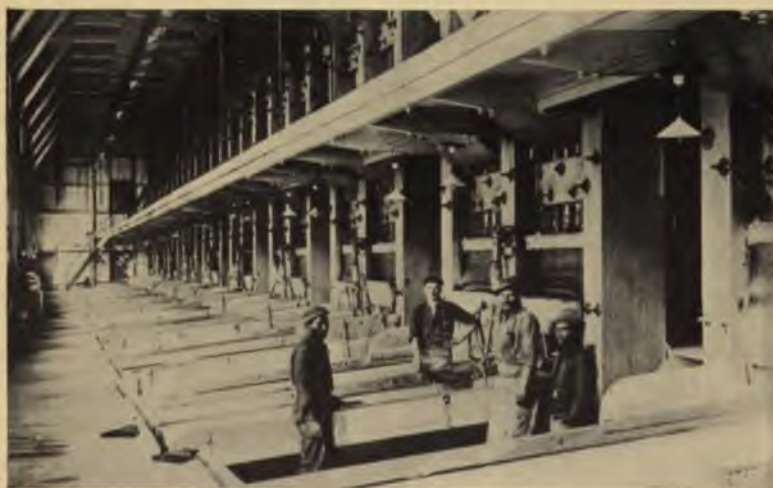
THE BATTERY, SHOWING THE MERCURY-COATED PLATES
